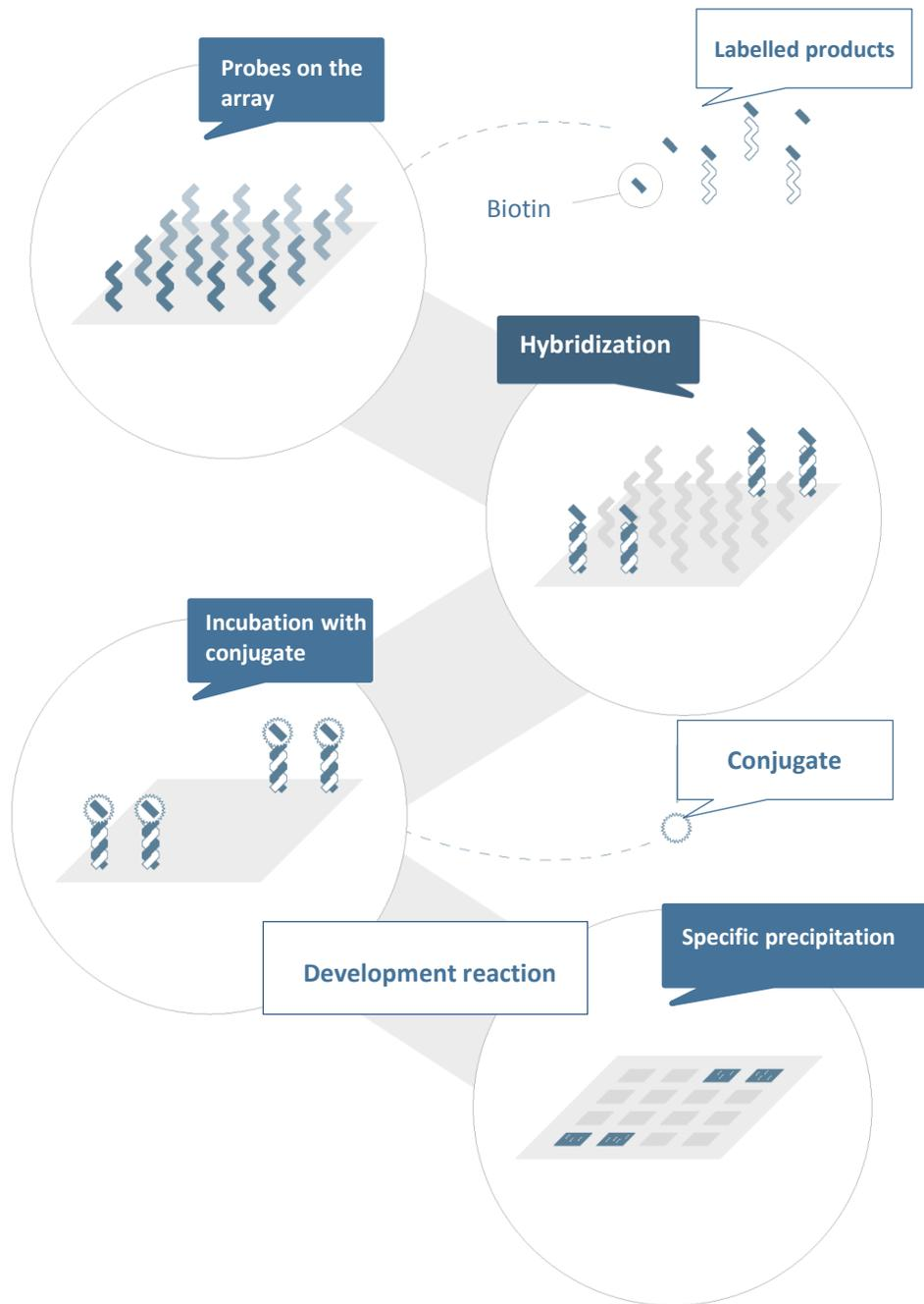
**Figure 2. Scheme of the detection system.** Probes immobilized on the microarray surface, capture complementary biotin-labelled amplified products. Subsequent binding of biotin to the streptavidin-peroxidase conjugate takes place. Finally, incubation with the peroxidase substrate o-dianisidine, yields a precipitate in the area where hybridization has occurred.
