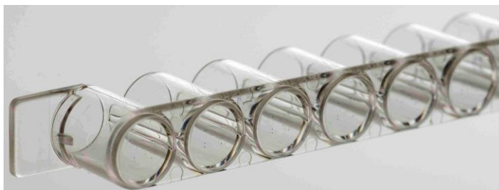
Figure 1. CLART-Strip®-CS platform in the form of an 8-well strip.
